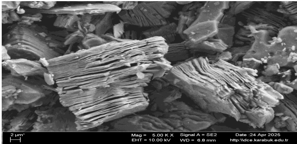
Figure.1. Scanning electron microscopy (SEM) image of \text{Ti}_3\text{C}_2\text{T}_x type MXene obtained by HF etching.
