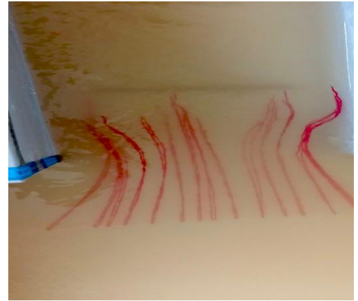
Fig.2. Formation pattern of the vortical flow field in the converging approach channel model.
